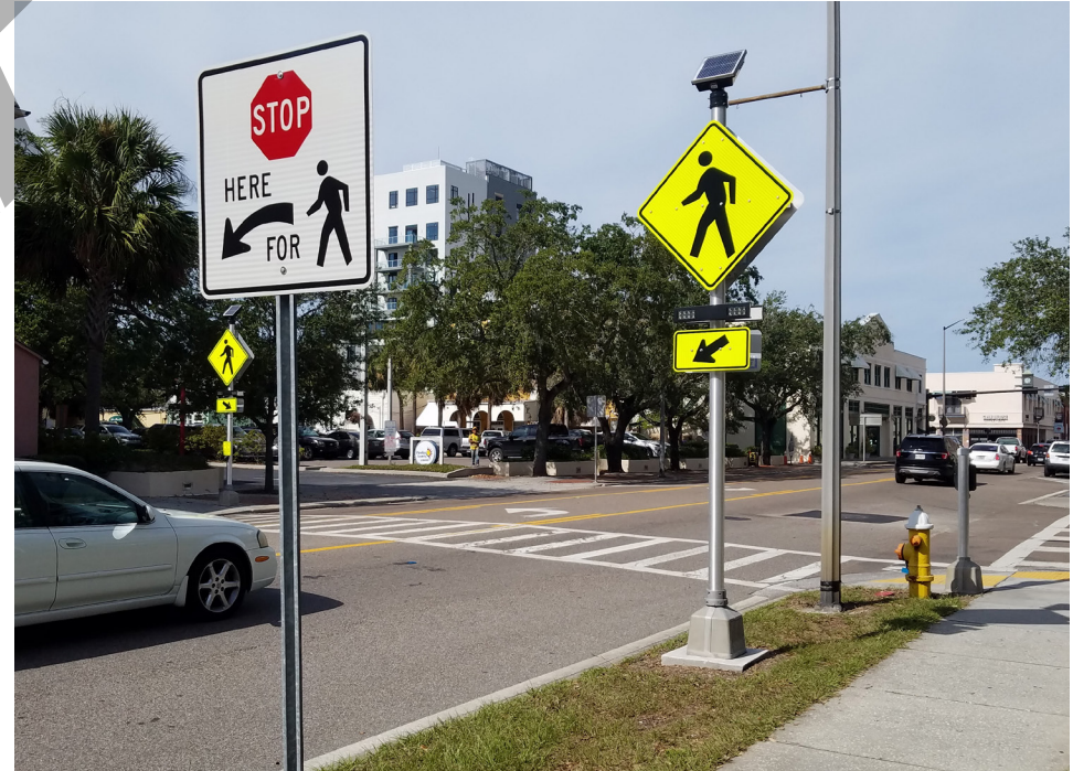
Crosswalk with a Rectangular Rapid Flashing Beacon (RRFB)
