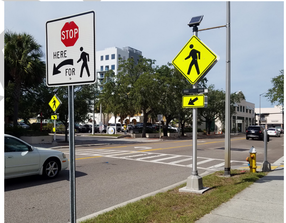
Crosswalk with a Rectangular Rapid Flashing Beacon (RRFB)
